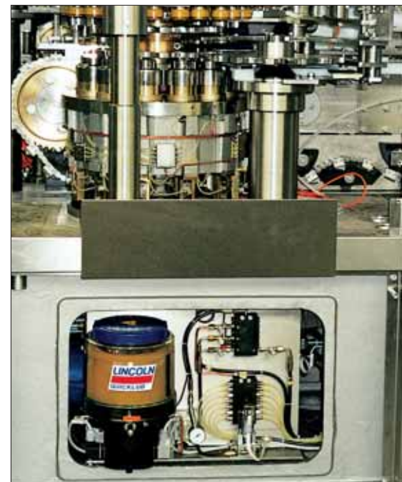
Filler with a Quicklub Progressive System
